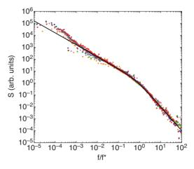
FIG. 5. (Color online) Master curve of all the power spectra. The horizontal axis has been scaled by the turnover frequency  $f^*$ . The line is a fit to Eq. (2).
