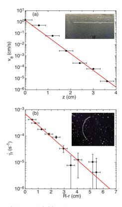
FIG. 2. (Color online) (a) Azimuthal velocity  $V_{\theta}$  at the outer wall as a function of depth below the surface z. (b) Radial shear strain rate  $\dot{\gamma}_r$  measured along the bottom plate of the system as a function of distance from the wall, R-r. Lines are fits to the data. Insets show representative traces of a single particle moving for 2 min along the sidewall (a) and for 20 min along the bottom plate (b), superimposed on snapshots of the whole field of view.
