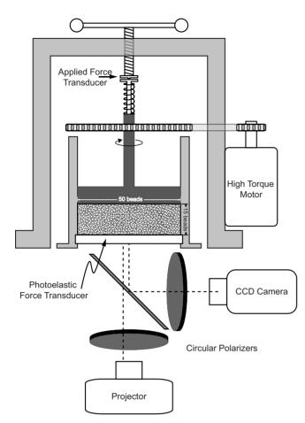
FIG. 1. Schematic diagram of the force-fluctuation measurement apparatus.
